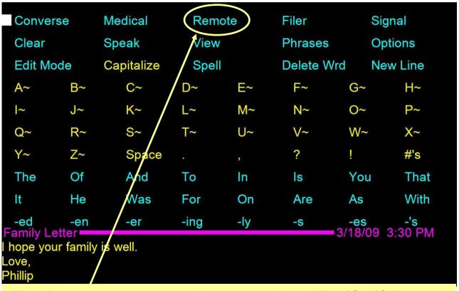
The Remote menu provides control of a TV (On/Off, Channel, Volume) or X10 modules (light, remote alarm).
